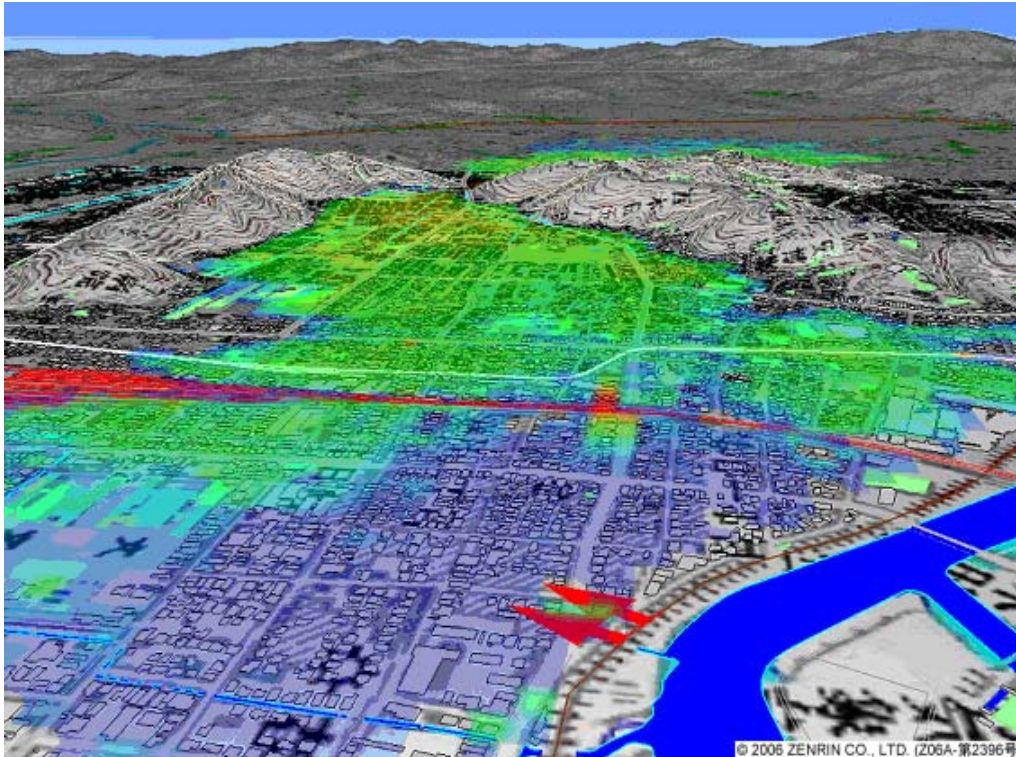
FIGURE 5. Enlarged graphics near the levee failure point indicated by red arrows. Simulated water depths are also shown (blue = 1 cm, green = 1 m, red = 4 m).
